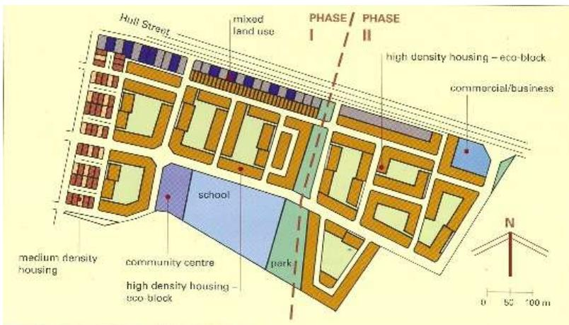
**Figure 7: Eco-blocks plan of Hull Street**
