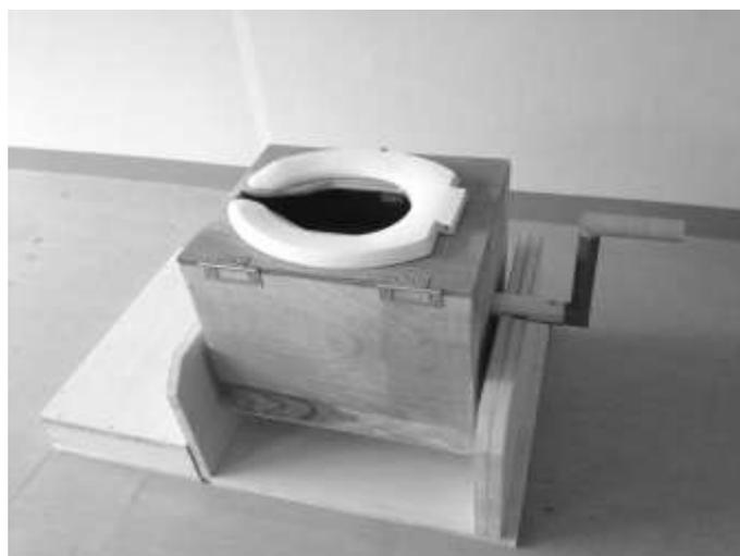
**Figure.2** The composting toilet we designed
