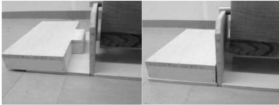
**Figure.3** Rotation stopper. Free (left) and locked (right).
