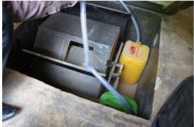
Figure 9. The composting reactor and tanks under the platform
