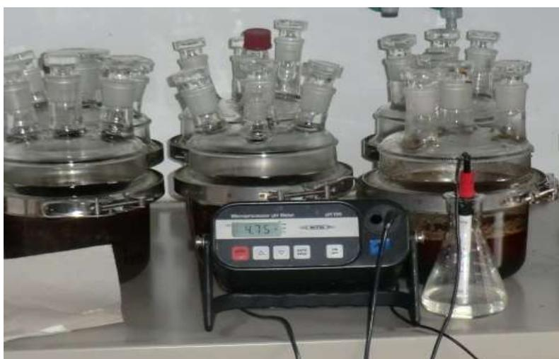
Figure 1: Fermentation reactors for batch LAF experiments
