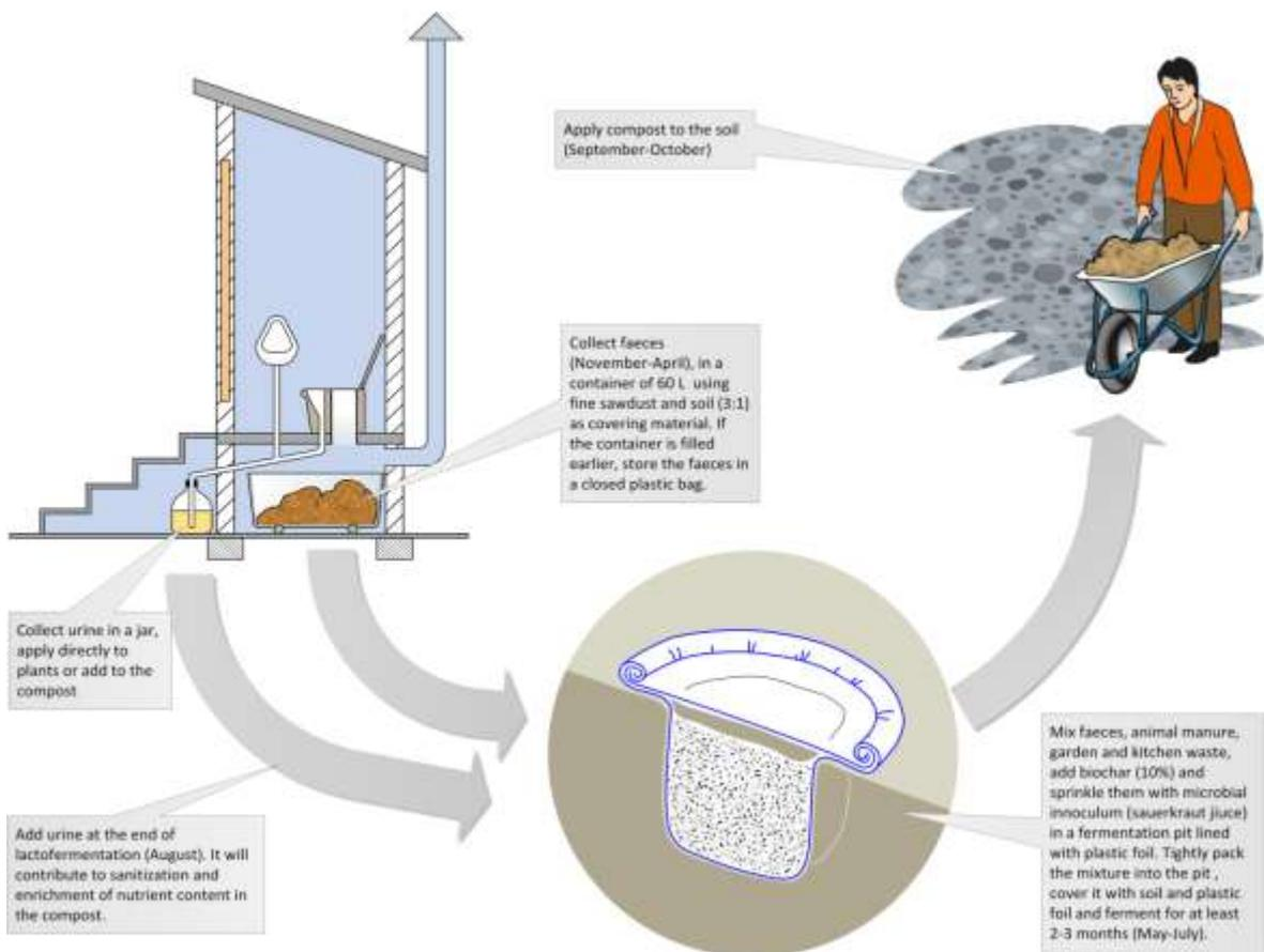
**Figure 2** Main principles of TPS approach carried out in an UDDT system at household level (adapted from Gensch, 2010)
