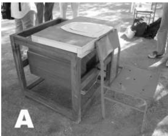
Fig. 2 Composting toilet (A) and slanted soil system for greywater treatment (B)
