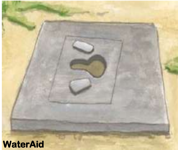
Traditional latrine (with concrete foundation slab)
